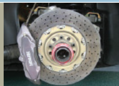
Example of carbon-carbon: the brake disc of this Ferrari race car's braking system is made from carbon-carbon.
