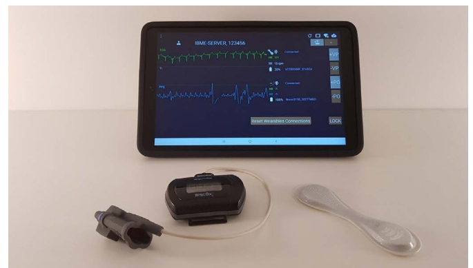
A wearable patch (to measure respiratory rate) and wrist-worn pulse oximeter (to measure pulse rate and oxygen saturation), are linked by Bluetooth to a tablet computer.
