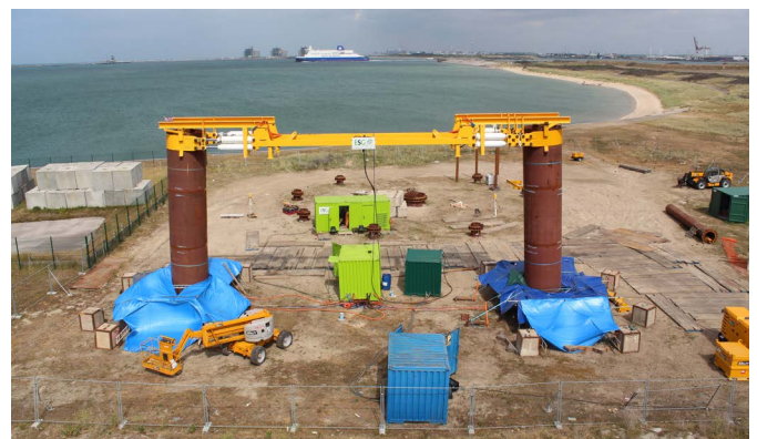
2.0 m diameter pile testing at Dunkirk in France
