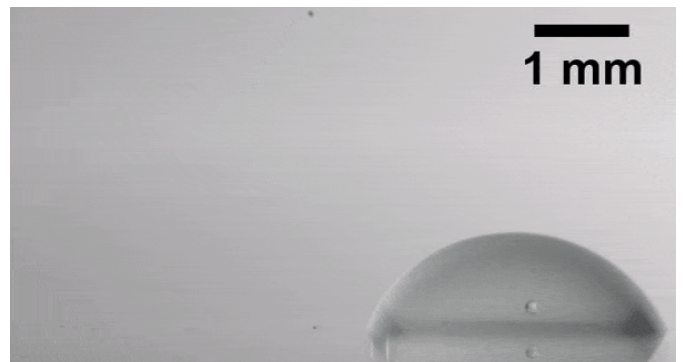
Two droplets of the same fluid combining as viewed from the side. From this viewpoint it is clear that the jet lies on the surface.
