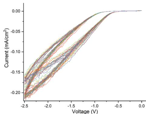
Figure S8 [continue]. Evolution of the CV curves of a DHTP@Zn-MOF-74 thin film sample subject to a total of 500 cycles at 50 mV/s. Panels (g)-(j) show cycles 301 – 500.
