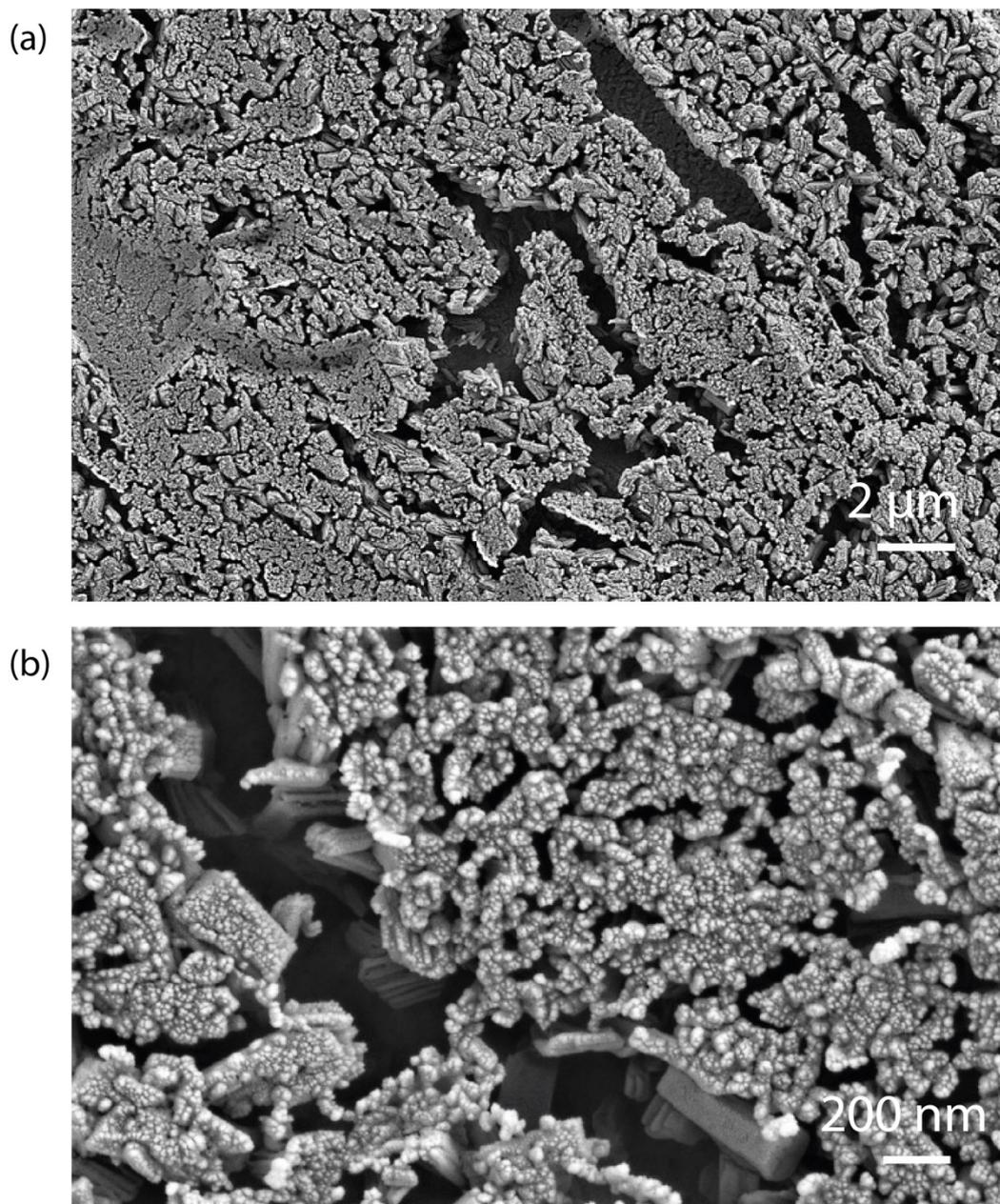
Figure S4. FESEM micrographs showing the nanoscale columnar-like morphologies of the DHTP@Zn-MOF-74 electrochromic film grown on the ITO-coated PET substrate (post-deposited with a layer of polycrystalline Zn, see Fig. S3).
