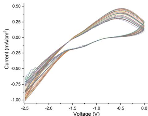
Figure S8. Evolution of the CV curves of a DHTP@Zn-MOF-74 thin film sample subject to a total of 500 cycles at 50 mV/s. (a) – (f) shows the first 300 cycles. Note that panel (a) is identical to data shown in Figure 4 in the main manuscript.
