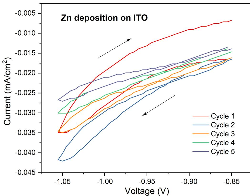
Figure S2. Zinc coating (grain size ~50 nm) deposited on the surface of ITO (on PET substrate) using the cyclic voltammetry (CV) technique. Five cycles were applied between -0.85 V to -1.055 V in a three-electrode electrochemical cell.
