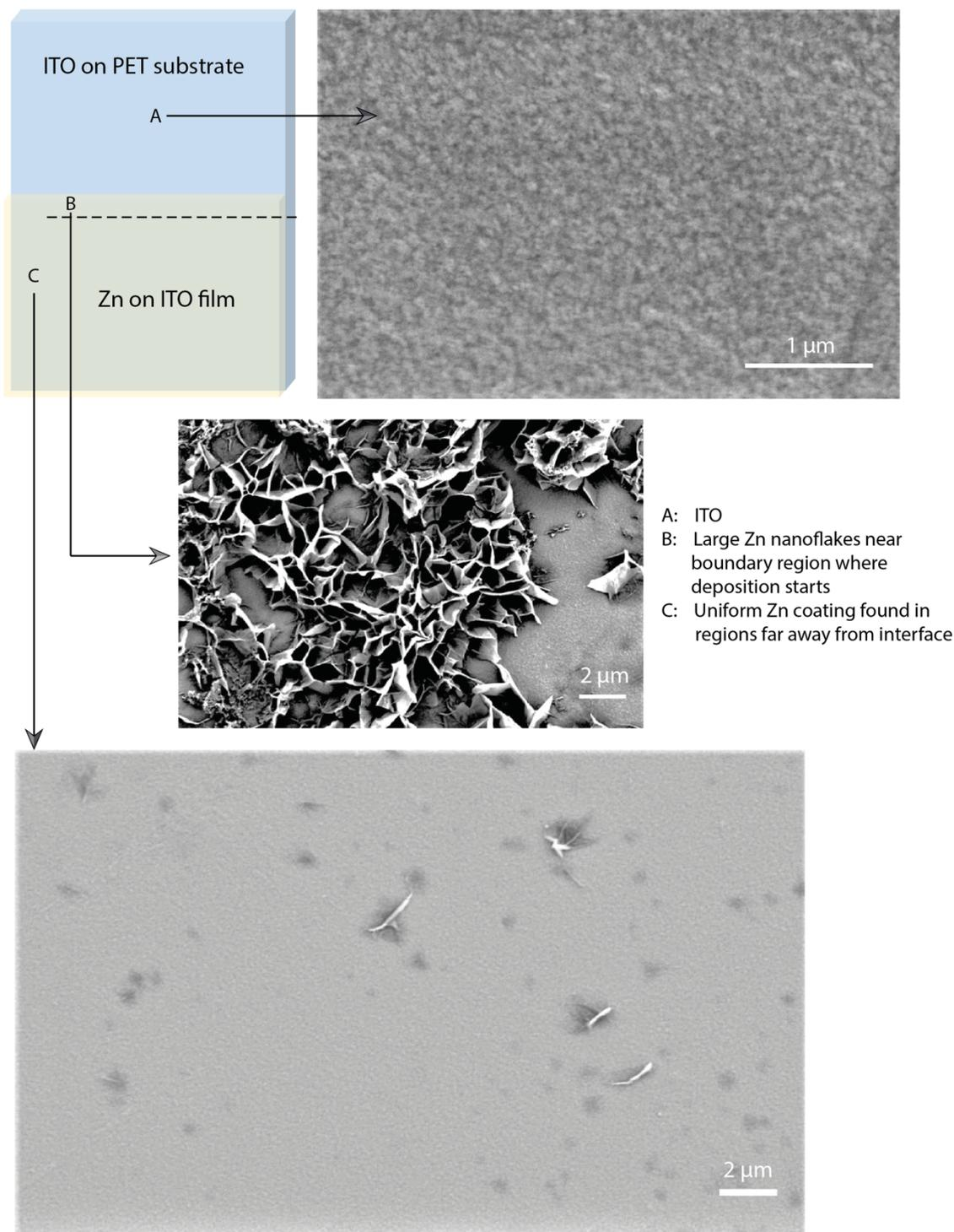
Figure S3. FESEM images showing the microstructures of Zn deposited on the ITO coated PET substrate. Note that the regions located in the vicinity of the liquid interface exhibit a non-regular flake-like microstructures due to the edge effect. The Zn coating found away from the interface was found to be more uniform.
