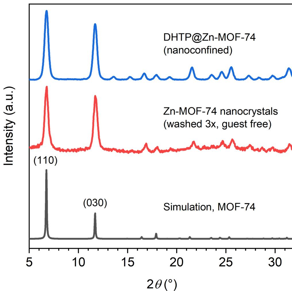
Figure S6. PXRD patterns of the as-synthesized nanocrystals (thoroughly washed to remove entrapped guests) and DHTP@Zn-MOF-74 sample compared to the simulated pattern.
