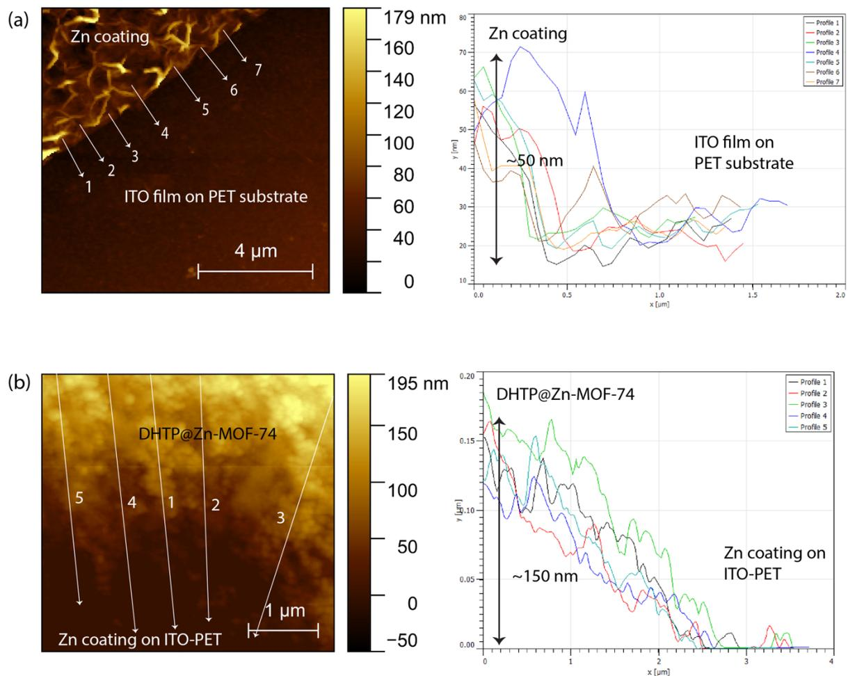
Figure S5. AFM height profiles across the (a) Zn to ITO interface, and (b) DHTP@Zn-MOF-74 to Zn interface.
