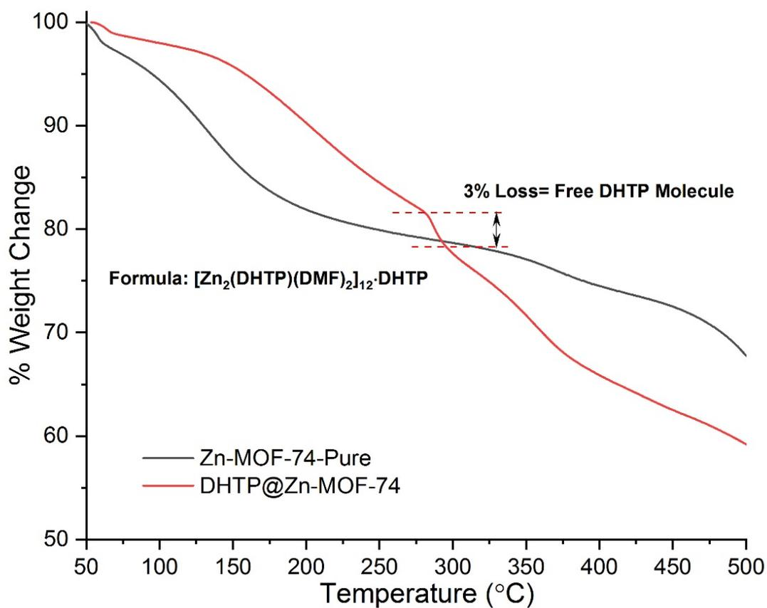
Figure S7. Thermogravimetric analysis curves for comparing the weight loss of the thoroughly washed Zn-MOF-74 versus DHTP@Zn-MOF-74 composite (a guest@MOF system) to determine the formula of the DHTP@Zn-MOF-74 compound as  $[Zn_2(DHTP)(DMF)_2]_{12} \cdot DHTP$ .
