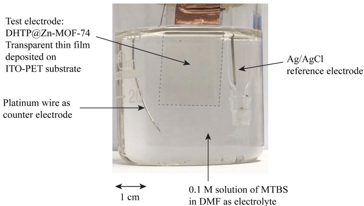
Figure S1. A three-electrode electrochemical test system for cyclic voltammetry. Ag/AgCl as the reference electrode, platinum as the counter electrode, and the transparent film of DHTP@Zn-MOF-74 as the test electrode. The clear electrolyte is 0.1 M tributylmethylammonium methyl sulfate conduction salt (MTBS) solution in DMF.
