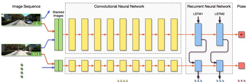
Following the architecture of Wang et al.<sup>1</sup>, the network is made up of a CNN pre-trained for optical flow<sup>2</sup> followed by an RNN.
