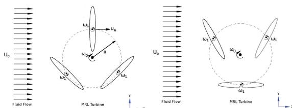
Fig. 1. MRL Turbine blade-position extremes
