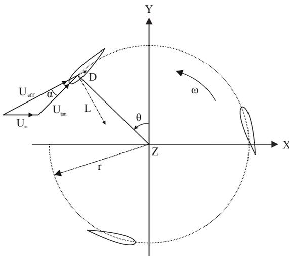
Fig. 1. Cross-section of a cross-flow tidal turbine
