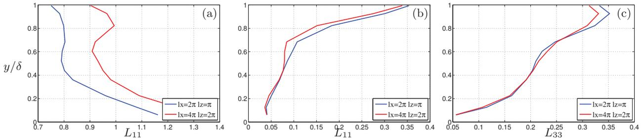
Figure 2: Turbulent lengthscales (a),  $L_{11}$  (streamwise) (b)  $L_{11}$  (spanwise) and (c)  $L_{33}$  (spanwise) for open channel flow with rigid lid at  $Re_t = 150$
