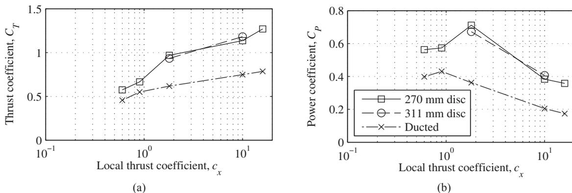
Fig. 2: Experimental measurements of (a) thrust coefficient and (b) power coefficient for ducted and unducted devices.
