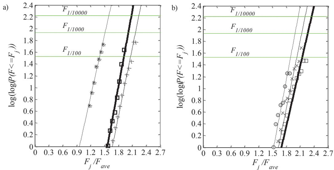
Figure 1: Extreme load variation from analysis of a) measured thrust due to turbulent flow and waves for a rigid structure ( $\omega_n = 85$  rads/s). Waves of wavelength  $9h$  (□),  $7.2h$  (+) and turbulent flow only (\*) b) predicted response based on measured kinematics of waves with wavelength  $9h$  opposing uniform flow. Natural frequencies of  $85$  rads/s (□),  $38.3$  rads/s (x) and  $27$  rads/s (○).
