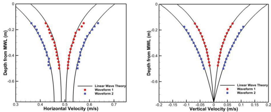
Figure 1 - Horizontal & vertical water particle velocities for both waveforms
