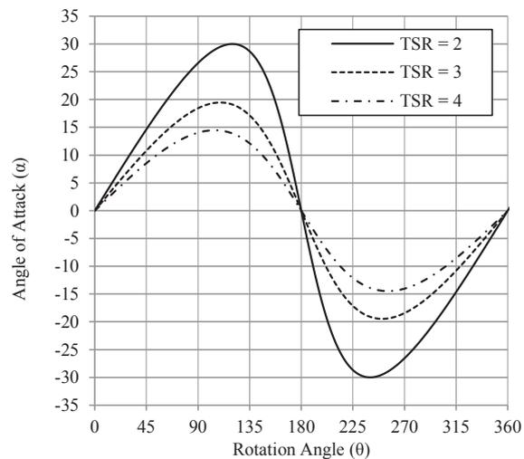
Fig. 2. Graph of angle of attack with rotation position
