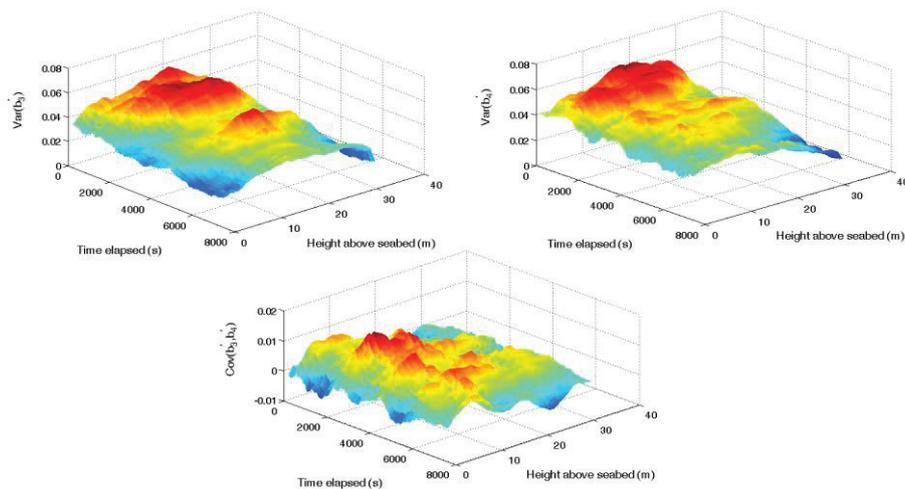
**Figure 1: Top two panels show variance in squares of velocity fluctuation for beams three and four; lower panel shows cross-beam covariance of the same quantity. Data is taken from site three, duration of data record is approximately one hour.**
