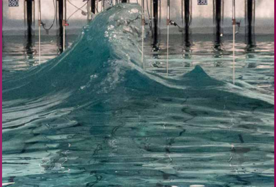
The laboratory recreation of the Draupner wave. Image: McAllister, M.L. et al. J. Fluid Mech. (2019); CC BY 4.0
