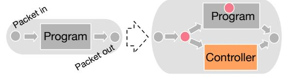
**Figure 4.** Transformation of the program to include a controller. Normal packets are handled as normal, but *direction packets* are passed to the controller. Pink dots represent *extension points*, one of which is added within the control flow of the original program in this illustration.
