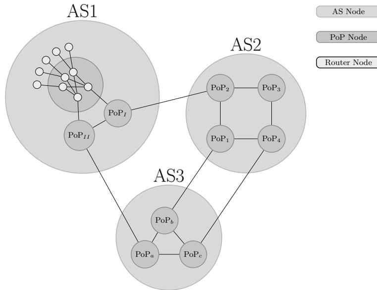
**Fig. 1.** The Internet's Levels of Aggregation
