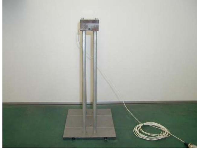
Figure 3.9: Test pile used in the centrifuge tests.
