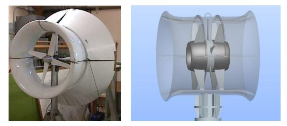
Figure 2.1: Examples of uni- and bidirectional ducts. Left: Vortec unidirectional duct for wind energy application (Phillips *et al.*, 2005). Right: CleanCurrent bidirectional duct for tidal energy application (Clean Current Power Systems Inc., 2013).
