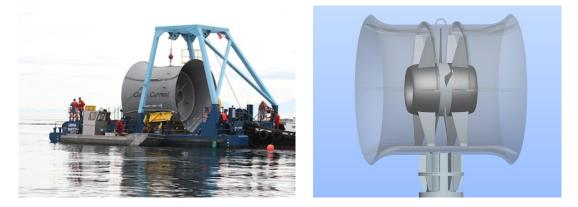
Figure 2.4: A 2006 (left) and 2010 (right) design version of the Clean Current tidal turbine by Clean Current Power Systems Inc. (2013).
