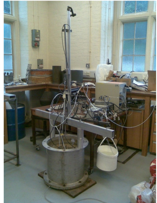
Figure 3.5.2. Photograph of the installation apparatus with Caisson 2 attached.
