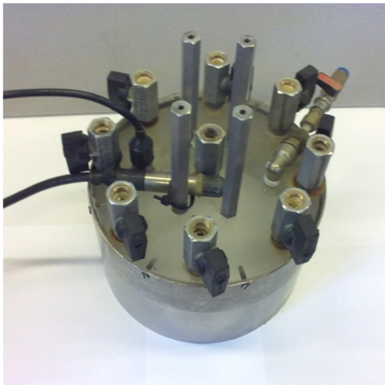
Figure 6.2.2. Photograph of Caisson 6 used for the grouting experiments.
