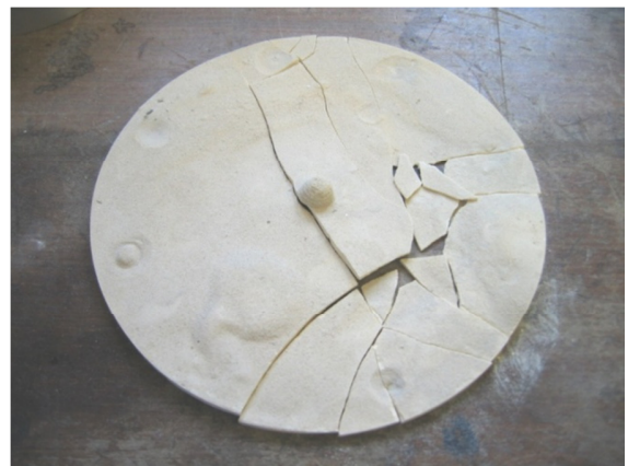
Figure 6.2.4. Photograph of grout disc removed from caisson. The visible surface is the side in contact with the soil. The protruding grout bulb in the centre of the caisson arose from sand scour where suction had been applied to the interior of the caisson for installation.
