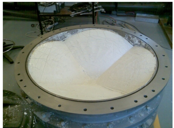
Figure 4.1.4. Photograph showing the inclined clay surface before the placement of sand.
