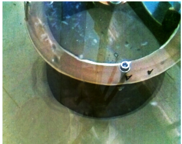
Figure 4.6.9. Photograph showing sand disturbance caused by failure of the clay layer beneath. The disturbance caused to the sand can be observed at the left of the caisson where the depression extends to the skirt. A small depression can also be observed at the right hand side of the picture.
