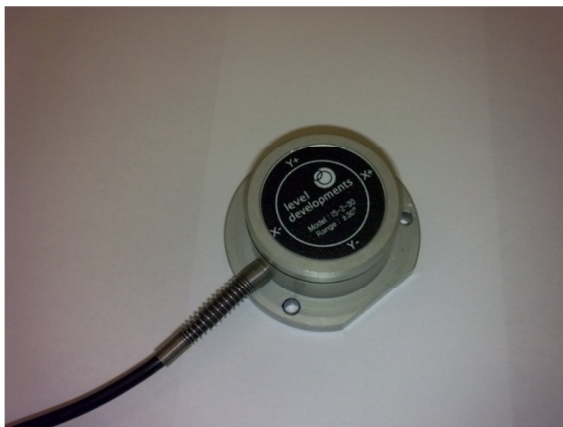
Figure 5.1.2. Photograph of inclinometer illustrating the small size packaging of the instrument.
