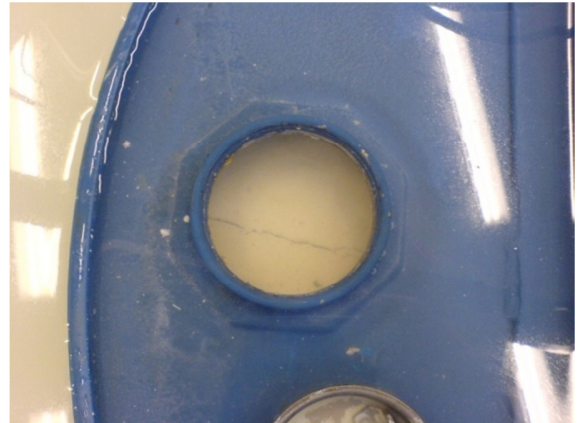
Figure 4.4.3. Photograph of Caisson 5 with lifted plug visible through aperture created by bung removal.
