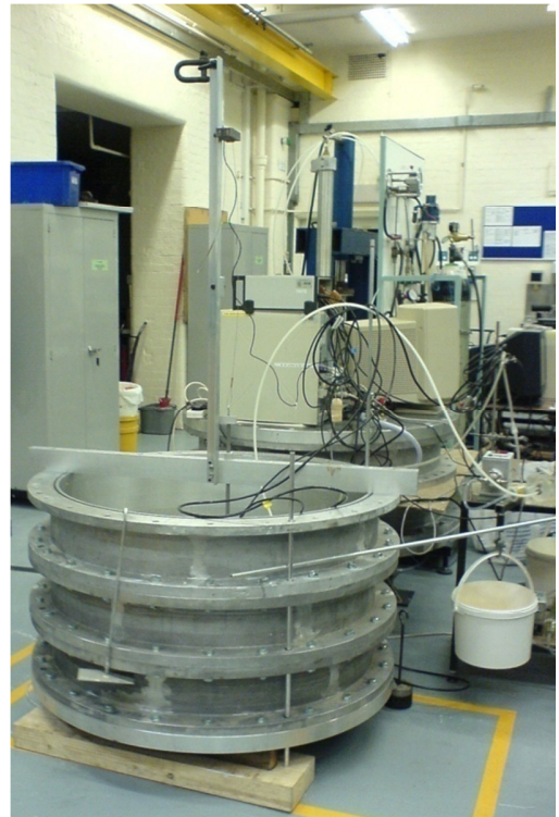
Figure 4.1.8. Installation apparatus used for layered soil tests.
