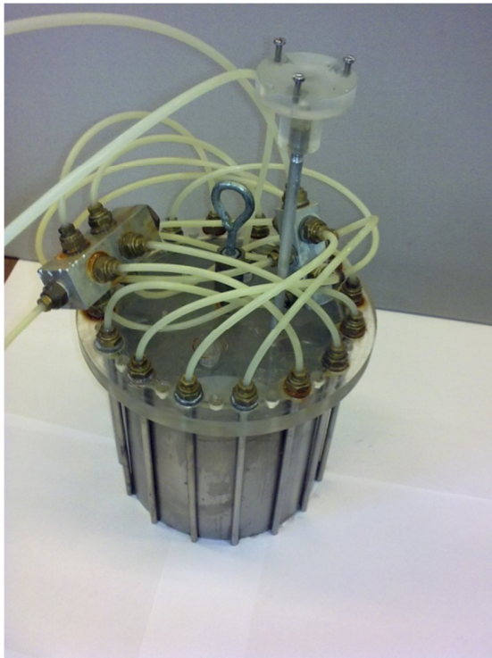
Figure 5.1.1. Photograph of caisson capable of skirt tip injection. The tubes running down the side of the skirt supply high pressure water to the nozzles at the ends.
