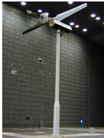
**Figure 4.2:** Wind turbine used in the NREL Phase VI wind tunnel experiments. [113].
