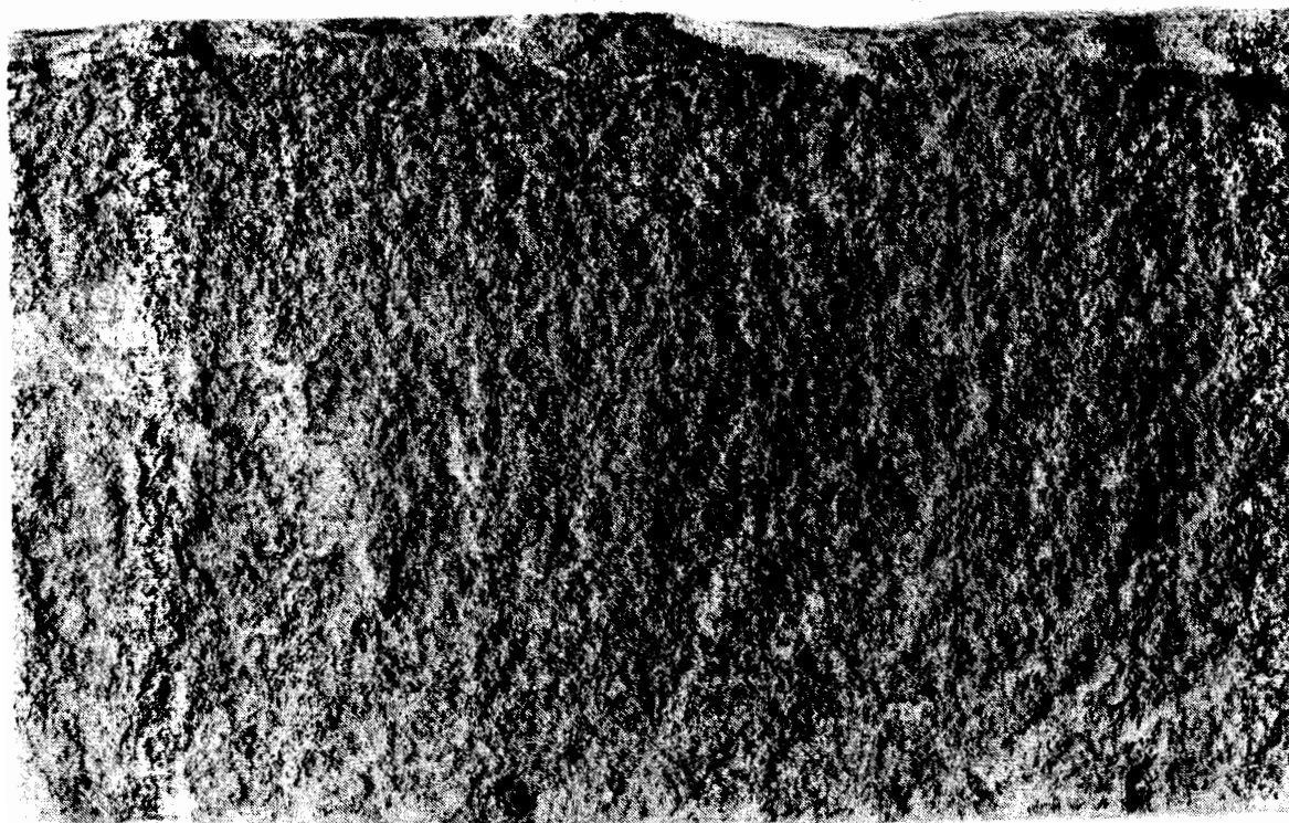
Plate 2.1 Appearance of Gassy Soil. Magnified x 6 Degree of Saturation = 0.8, 1-D Consolidation to 35 kPa (Nageswaran, 1983)
