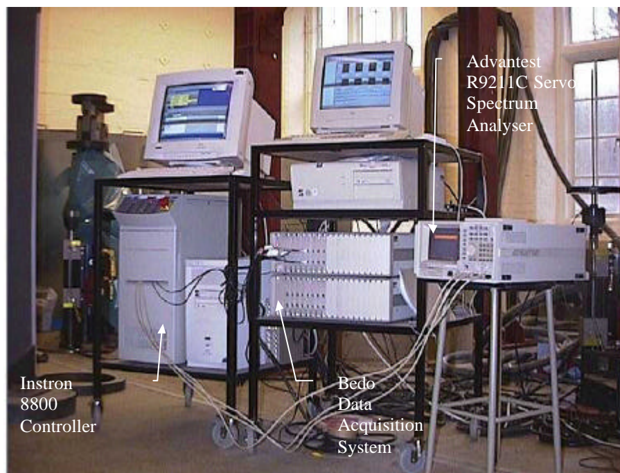
Figure 30. The Instron 8800 Controller, Bedo Data Acquisition System and Advantest R9211C Servo-Spectrum Analyser
