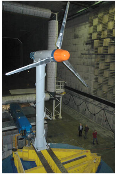
Figure 3.1: Photograph of the MEXICO rotor in the Large Low-speed facility (LLF) of the German-Dutch Wind Tunnels (DNW) in December 2006 (Schepers et al. 2012).
