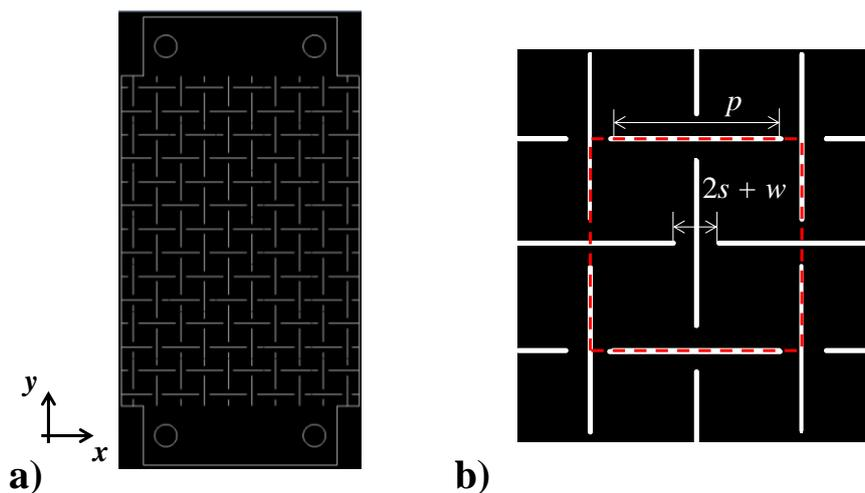
Figure S1: a) Laser pathway for the design of the metamaterial sheet, including the upper and base regions which are clamped to microtensile loader and b) parameters defining the lattice dimensions of the system. The red line marks the representative unit cell of the system.
