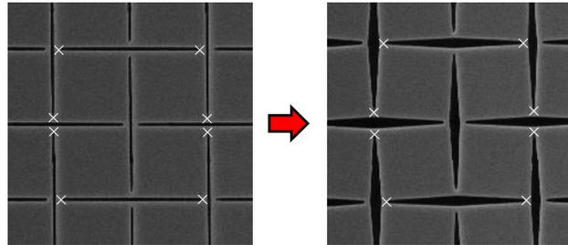
**Figure S3: Images of the FIB-milled system with markers indicating the regions of the system which were tracked during the point tracking analysis. The same technique was used for the rubber and Kapton macroscale metamaterials.**
