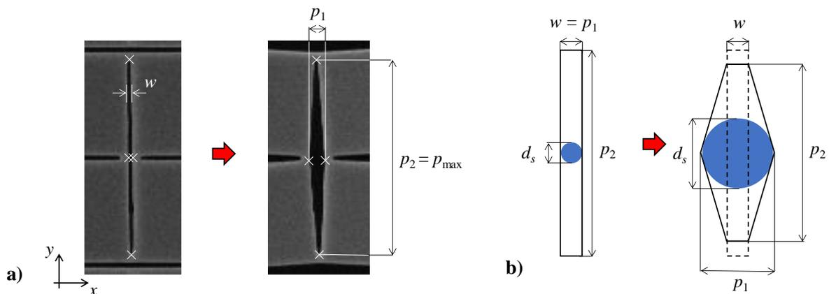
**Figure S5:** a) Image of tracked pore points in SEM images and b) a sketch showing how the spherical porosity of the system changes with increasing strain.
