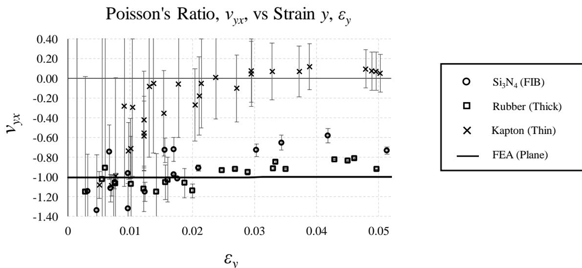
**Figure S4: Poisson's ratio vs Strain for each data point with standard deviation (equivalent of Figure 2d in main manuscript).**
