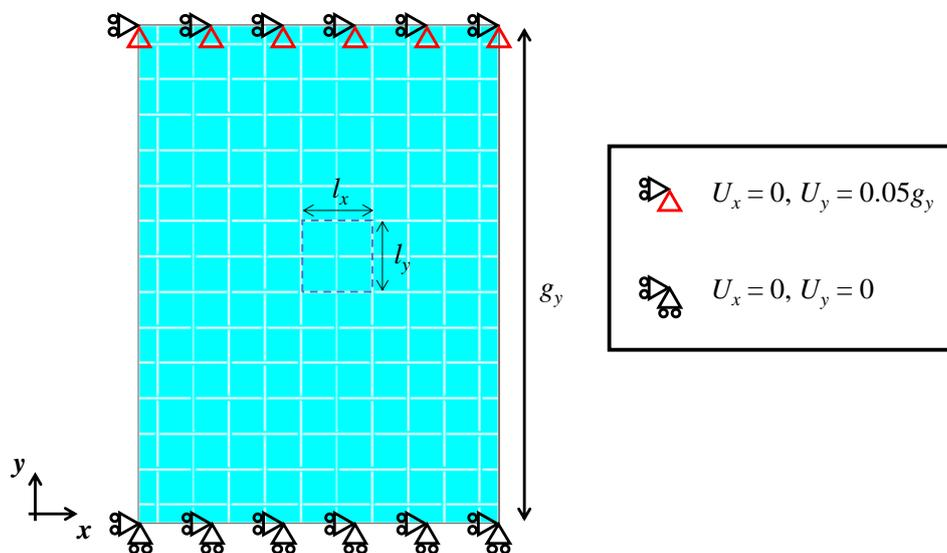
**Figure S2: Fixes and loads applied to the FE system and a marked region indicating the section from which the Poisson's ratio of the central repeating unit was measured.**
