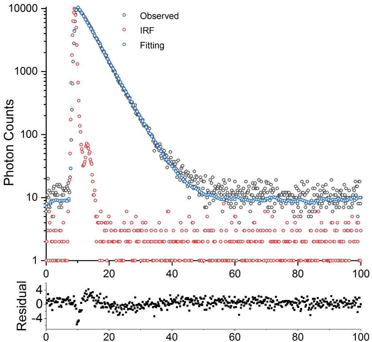
**Figure S9.** Lifetime decay profile of A+B@ZIF-8 powder measured for the emission maximum at 577 nm.
