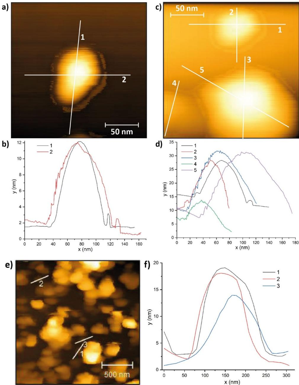
**Figure S5.** Representative AFM images of the nanodiscs of A+B@ZIF-8 (top, a & c), with a graph showing their height profiles (bottom b & d) extracted from the marked regions of the nanodiscs. The nanodiscs exhibit an aspect ratio (width/height) ranging from 5:1 to 10:1
