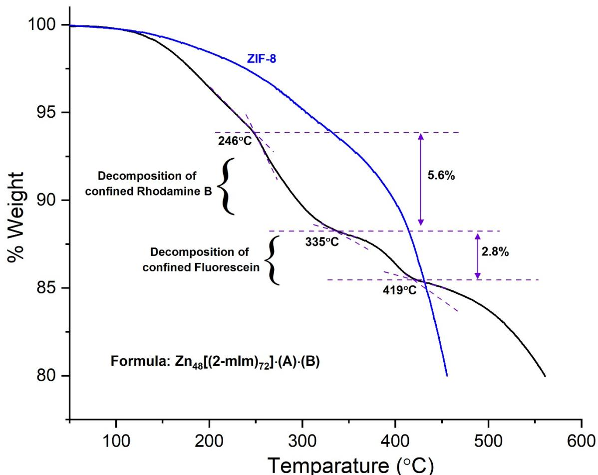
**Figure S6.** TGA of A+B@ZIF-8 powder indicating stepwise degradation of the two confined guest species: Rhodamine B and Fluorescein (A), which were estimated to be at 5.6 wt.% and 2.8 wt.%, respectively. TGA of pristine ZIF-8 is shown for comparison, which was synthesised using the same conditions to that of A+B@ZIF-8 (but without the addition of A+B guest solution).
