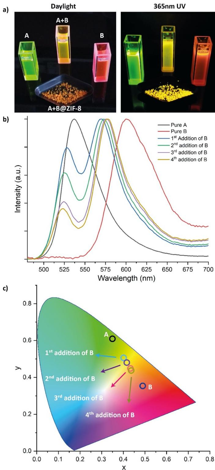
**Figure S2.** (a) Photograph taken under the 365 nm UV lamp, showing the emission of solutions A = Fluorescein, B = Rhodamine B, A+B mixture, and the solid-state emission of A+B@ZIF-8 powder (after drying). (b) Changes in the emission spectra of the combined solutions of A+B upon addition of 300  $\mu$ L of B into A at each incremental point, (c) CIE 1931 diagram showing changes in colour chromaticity corresponding to the spectra in (b).
