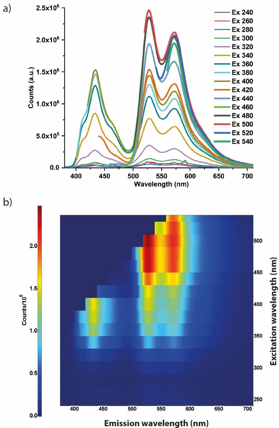
**Figure S4.** (a) Emission spectra of the 3D printed pellet (3 mm thickness) showing the unchanging emission wavelengths subject to different excitation wavelengths, ranging from 240–540 nm. (b) Excitation-emission map corresponding to the series of spectral data in (a). The measurements were performed using the FS5 spectrofluorometer.
