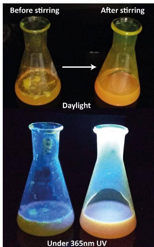
**Figure S3.** Photograph showing the effect of overnight stirring of (wet powder) A+B@ZIF-8 into the clear photopolymer resin, it was found that the non-homogenous mixture turned into a uniform homogenous suspension after overnight stirring.
