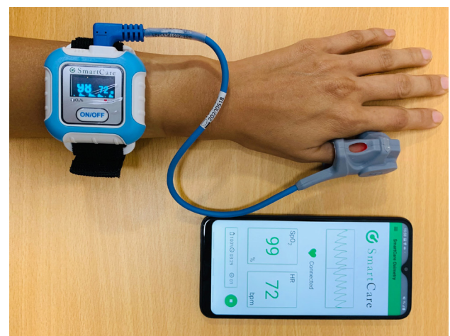
Figure 2 Wearable pulse oximeter device and smartphone display used for remote monitoring.
