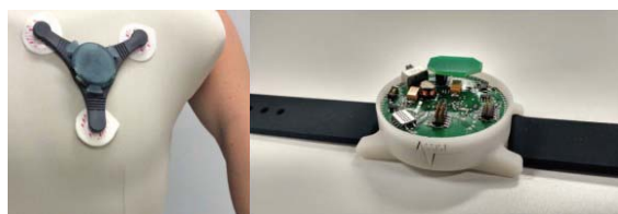
Fig. 5. Prototype for a chest patch and a wristband that can track vital signs and environmental factors [6].
