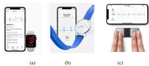
Fig. 2. Asthmatic monitoring using ECG. (a) Apple iWatch [58]. (b) Withings watch [59]. (c) KardiaMobile ECG monitor [74].
