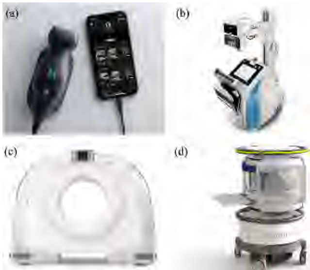
Fig. 10. Portable medical imaging devices (a) portable ultrasound system (Butterfly) [113], [176], (b) Optima XR220amx portal X ray (GE) [177], (c) BodyTom CT scanner (Samsung) [115], [178], and (d) portable MRI (Hyperfine) [166], [179].
