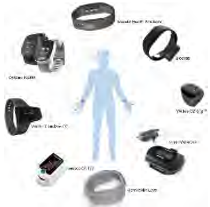
Fig. 2. Commercially available wearable pulse oximeters, Oxitone 1000M (Oxitone, Hartford, USA) [26], Checkme O 2 (Viatom, Shenzhen, China) [27], Timesco CN130, Loop (SpryHealth, California, USA), WristOx2 (Nonin Medical Inc, Plymouth, United Kingdom), Wellue O 2 Ring (Wellue Health, Shenzhen, China), Biostrap (Biostrap, California, USA), and Wavelet Health Wristband (Wavelet, California, USA).
